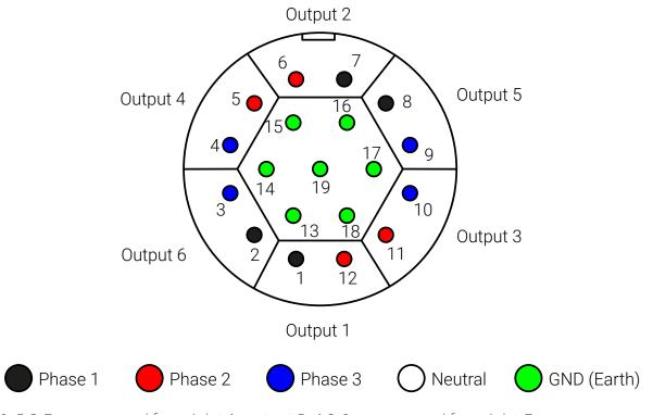
Outputs 1, 3 & 5 are powered from inlet A; output 2, 4 & 6 are powered from inlet B.
