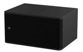
The Venu 215 V2 is a double 15" reflex-loaded low frequency enclosure, providing a frequency response of  $38 \text{ Hz} - 160 \text{ Hz} \pm 3 \text{ dB}$  and efficiency of 101 dB. Features include tough 15" high excursion transducers with 4" voice coils and a durable enclosure made entirely from 18 mm multi-laminate birch plywood.
