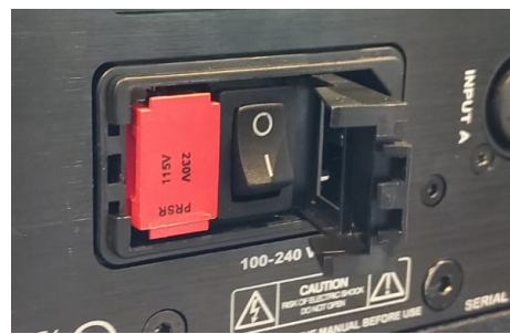
Step 4: Insert the fuse holder ensuring it is fully engaged.
